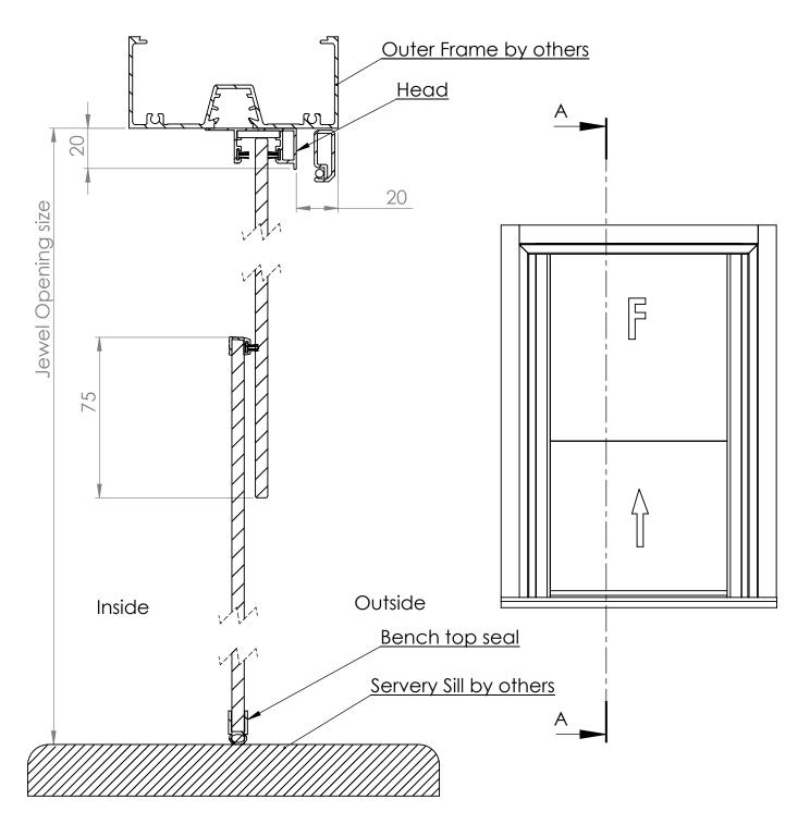
Note: this sill is not water ratted This window should be installed with some weather protection
